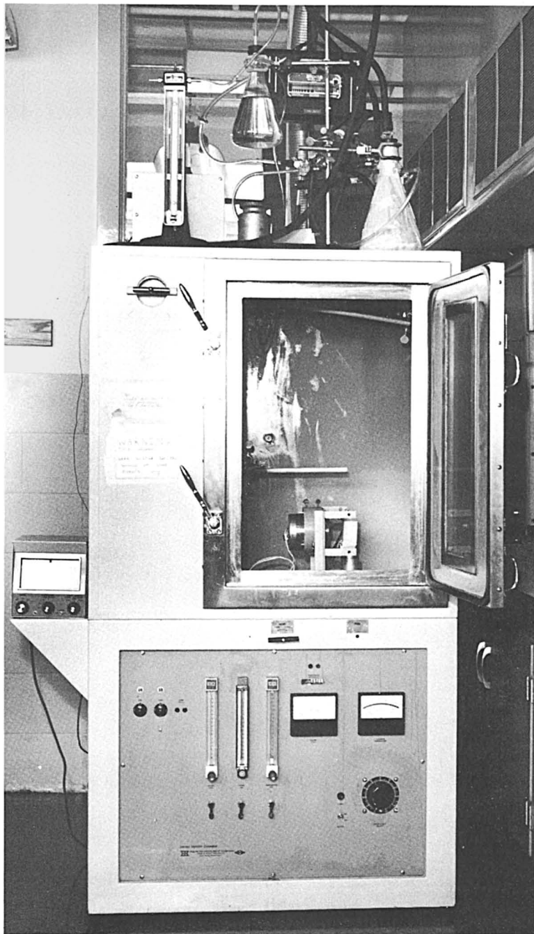
Figure 7. NBS smoke chamber is used to determine the obscured optical density from various materials.
