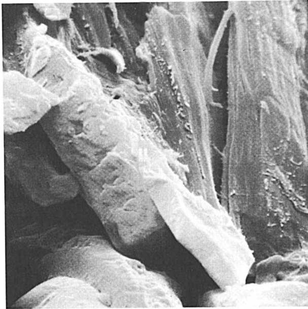
Figure 10. Scanning electron micrograph of a composite of cellulose powder-lignin powder mixture. The big, fibrous cellulose particle (right) appears to be bonded to the big amorphous lignin particle (left). A split in the cellulose particle suggests that bonding between lignin and cellulose particles was stronger than the tensile strength of cellulose perpendicular to the fiber axis (124).
