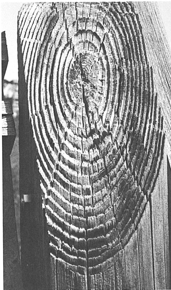
Figure 8. Weathered surface of softwood after 15 years of exposure (in Madison, Wisconsin).
