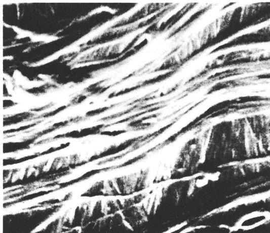
Figure 10. Photomicrograph of delignified cell-wall softwood fibers ( \times 16,000 ).
