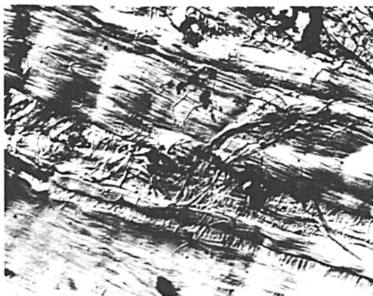
Figure 9. Photomicrograph of softwood fiber embedded in lignin ( \times 4000 ).
